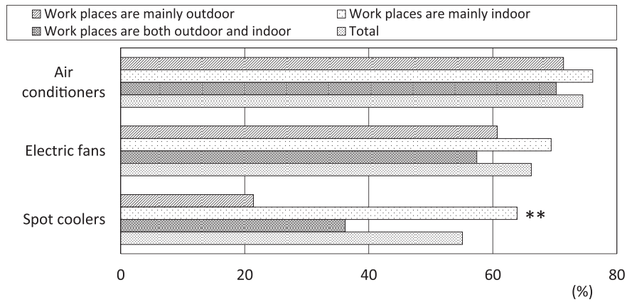
Fig. 2 Setting situation of air conditioners, electric fans and spot coolers in the working places among three groups of enterprises with 50 or more workers. Significant differences among the three groups; * * p < 0.01 .
